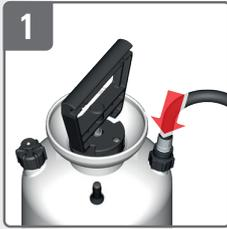
**1** Screw hose onto pressure tank
