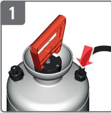
**1** Screw hose onto pressure tank
