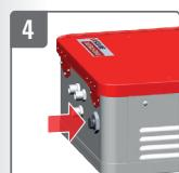
Insert the cleaned filter completely
