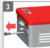
Remove the filter and clean/replace
